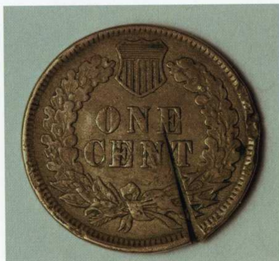
Copper-nickel 1890 Indian Cent with a test cut/
